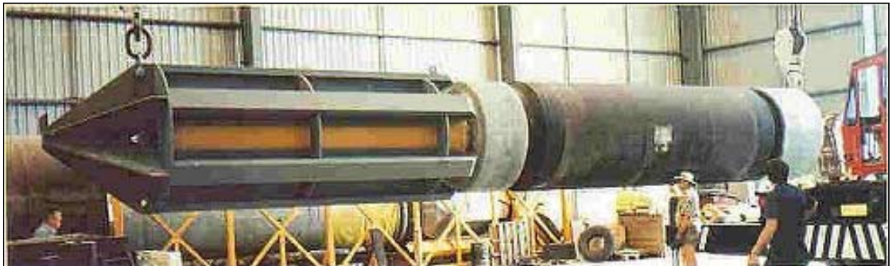
Figure 6 - Pile reforming Packer (1.8 m diameter x 6 m long rated for 2000 psi )
